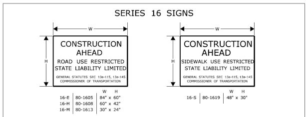
THE 16-S SIGN SHALL BE USED ON ALL PROJECTS THAT REQUIRE SIDEWALK RECONSTRUCTION OR RESTRICT PEDESTRIAN TRAVEL ON AN EXISTING SIDEWALK.
